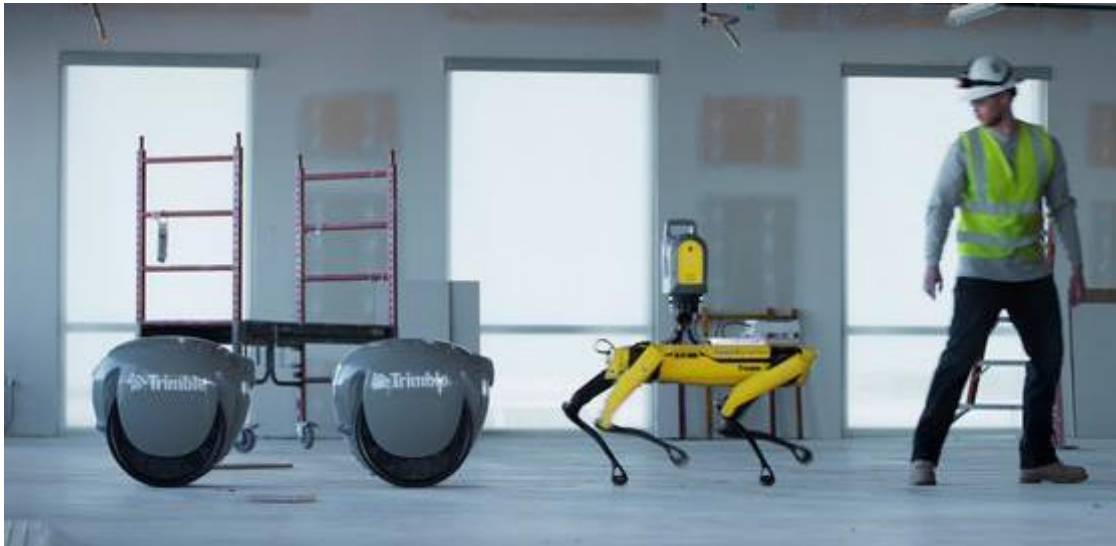
PFFtag™, smart following module prototype, onto a Boston Dynamics' Spot® robot controlled by Trimble's advanced positioning technology
